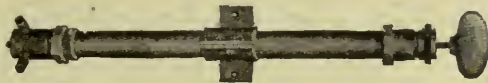
FIG. 373.—Hand water pumps for use with flash boilers. It is intended to be placed in front of seat, between the two passengers. The bracket in center being movable, enables the pump to be placed at any height to suit the car. The water connections are for one-quarter inch pipe. The plunger is quite small as the resistance to be overcome—that due to the high working pressure of the flash boiler—is considerable, in fact it would be too great for hand operation if the plunger were large as shown in fig. 372.
